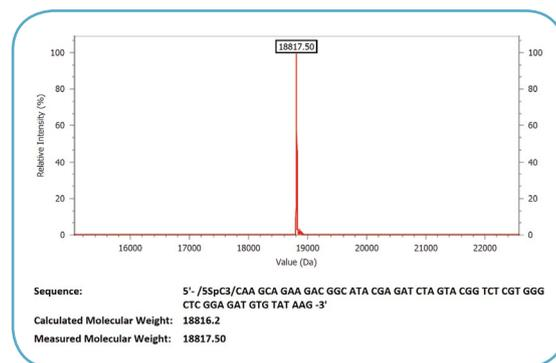
**Figure 3.** ESI mass spectrogram of an HPLC-purified, 60 nt oligonucleotide with a 5' spacer modification. The synthesized sequence is shown at the bottom and the expected and observed molecular weights (Da) are presented above the sequence.
