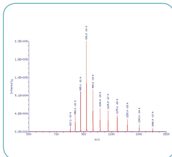
**Figure 2. ESI mass spectrometry trace (raw data) of an HPLC-purified, 60 nt oligonucleotide with a 5' spacer modification.** Multiple peaks are seen at different m/z ratios, representing various amounts of deprotonation.
